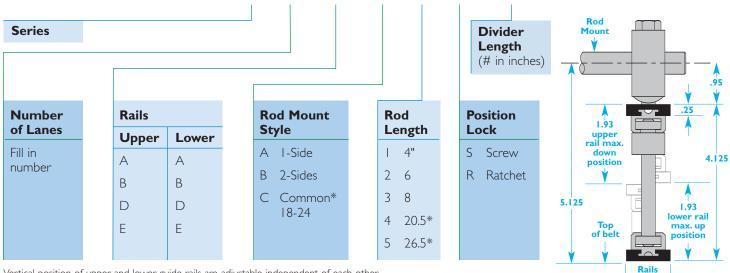
Vertical position of upper and lower guide rails are adjustable independent of each other.
