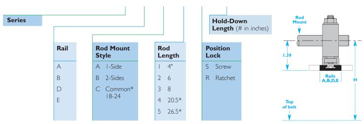
\* Common "C" type rod mounts are intended for only 18"-24" conveyors. Each rod requires (2) #2077 cross blocks.
