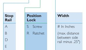
Note: end stop will function on side rails "A" through "E." Stop can be positioned along length of side rail.
